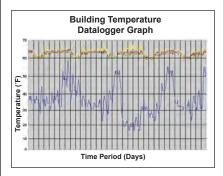
Building studies show small blow-thru type space heaters reduce stratification with their high velocity vertical throw diffusers. They achieve 3°F to 5°F temperature variation, which is the same or better than large air turnover systems while using much less energy.
