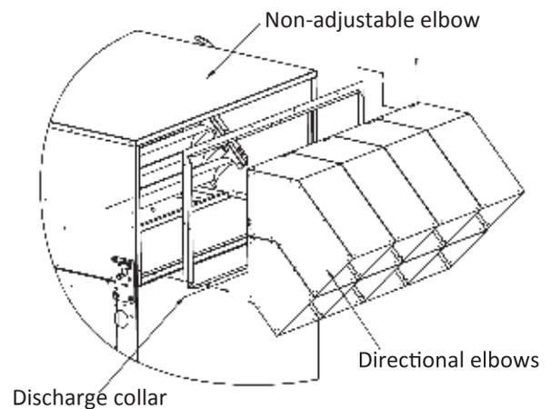
6. Seal all seams between heater and accessories using appropriate contractor grade caulk to mitigate potential water ingestion and pressure loss.
