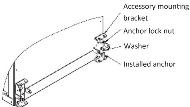
9. Continue attaching discharge accessories to heater as needed using the provided mounting brackets.
