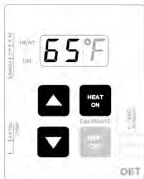
2. Press and hold the **HEAT OFF** button while pressing the **UP** or the **DOWN** button until the desired temperature for the heater to turn OFF is displayed.
