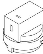
This gas pressure switch is a manual reset safety device to lock out the burner operation should large gas pressure fluctuations occur. The high gas pressure switch should be set 3" WC above manifold gas pressure. The low pressure switch should be set at 2" WC. The adjustment screw is located under the top plate. The low gas pressure switch will have to be reset whenever gas supply has been interrupted.
