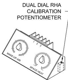
10. Allow the discharge temperature and manifold pressure to stabilize between adjustments until the manifold pressure and discharge temperature comply with the guidelines of the Calibration Check procedure step “8b” (page 57).
