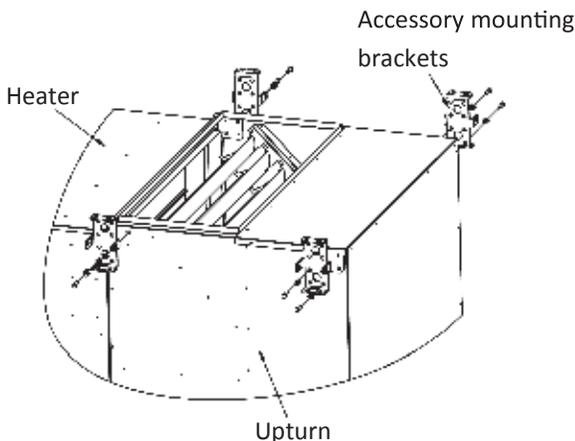
4. Lift the duct extension into place and secure it with the accessory mounting brackets removed in the previous step.
