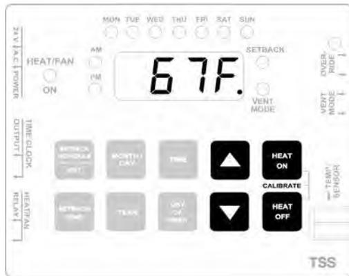
2. Pressing the **UP** or the **DOWN** button will display the current calibration difference above or below (-) the measured temperature.
