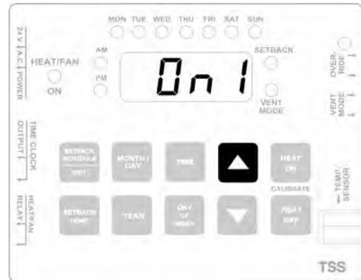
8. Press and hold the **TIME** button while pressing the **UP** or the **DOWN** button to scroll to the desired ON time.
