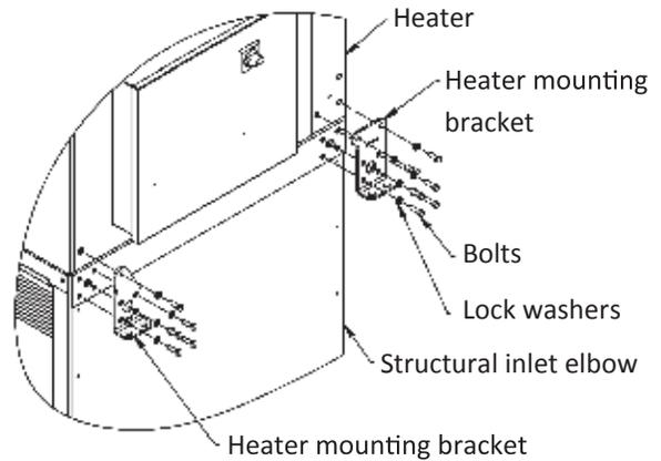
10. It is recommended to run support back to the wall to prevent swaying or tipping of heater and accessories.
