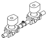
The leak test facility is provided on all heaters over 400,000 Btu/hr. It consists of a momentary switch for the shut-off valve (SOV) in the gas train and a gauge port between the (SOV) and (SSV) shut-off valve. By holding the gas valve momentary switch closed, the (SOV) gas valve is energized which allows gas pressure to build on the seat of the SSV safety shut-off gas valve. The gauge port between valves is
