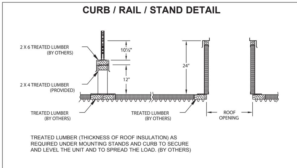
\* Dimensions allow for 3/4" clearance on each side
