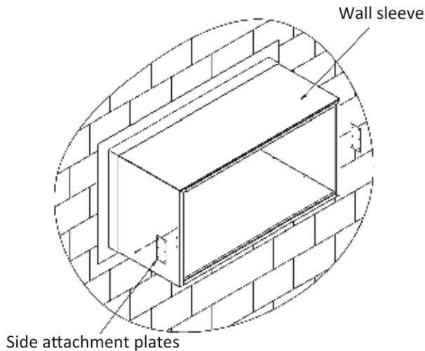
2. Lift the downturn with lugs into place and secure it using the retaining clip and side attachment plates.
