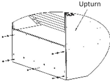
2. Lift the upturn into place on top of the 4' stand, being sure to catch the lip of the upturn on the unit's retaining clip. Replace the washers and nuts removed from step 1 onto the threaded PEM studs now inside of the unit and tighten securely.
