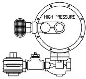
The HPR option is required when the gas supply pressure exceeds the nameplate rating for the heater.
