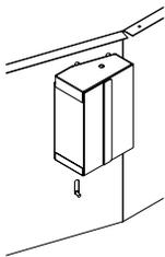
The discharge air temperature sampling box is located on the side of the discharge, and is accessible from the electrical control enclosure side of the unit. The sampling box houses the high limit (HL) and the discharge temperature sensor (DTS). This box should not be tampered with unless performing the Calibration Procedures (pages 60–62).
