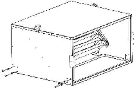
2. Prepare the upstream accessory or heater by removing the accessory mounting brackets.
