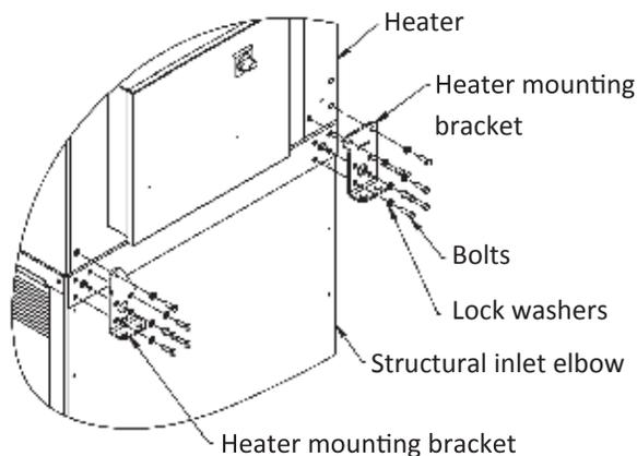
4. Continue attaching discharge accessories with provided mounting brackets as needed.
