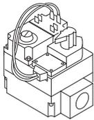
The combination valve serves as a manifold pressure regulator and redundant gas shut-off valve. This control is typically used for gas capacities below 400,000 Btu/hr. The valve operates on 24 Volts AC
