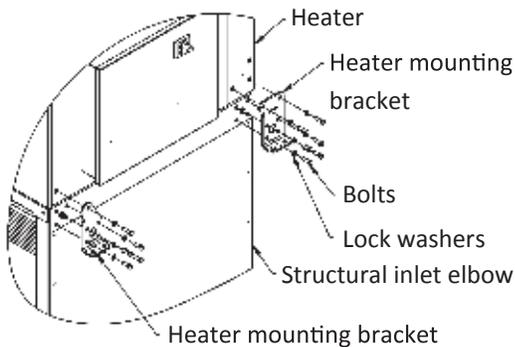
4. If not already attached, secure elbow to discharge of heater using provided heater mounting brackets.
