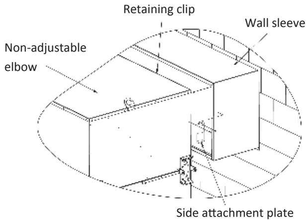
3. Use the appropriate framing techniques to frame, insulate, and flash the hole through which the wall sleeve is protruding.
