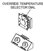
As discussed under the component description for the EDR control system, the RHA may have a single or dual adjusting knob(s) on the dial face. The single adjusting knob control permits manual adjustment of the discharge air temperature from 55 to 130°F. The override
