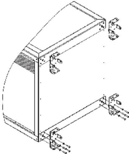
2. Determine the distance needed between the building wall and the heater.
