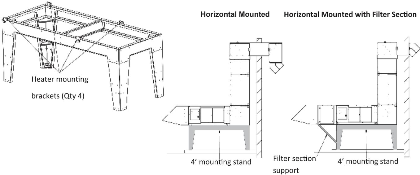
The horizontal S-Series mounting stand is suitable for outdoor pad mounted configurations. The 48" height is ideal for easy maintenance access while still remaining high enough to avoid potential snow ingestion from the ground during winter months. It is designed to be installed perpendicular to the building and includes room for both the unit and upturn to be situated on the frame. Additional support legs are provided if a filter section is ordered.
