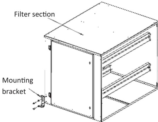
9. Lift the filter section into place at the inlet end of heater. Secure by resting filter section onto unit's retaining bracket while using self tapping screws to fasten the internal flange of the filter section the unit's front face.
