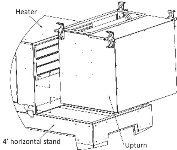
3. Remove the accessory mounting brackets on the upturn in preparation to attach the duct extension.
