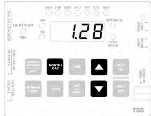
4. Press and hold the **YEAR** button while pressing the **UP** or the **DOWN** button until the current year is displayed.
