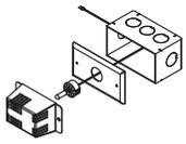
The thermistor is wired to the remote temperature sensor terminal block. If remote location of the sensor is desired, the connecting cable must be wired between the thermistor and this point.
