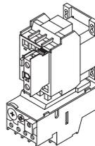
The motor starter assembly consists of a motor starter, overload relay and auxiliary contact. The overload relay protects the motor from excessive current or single phasing. If the overload relay trips, it must be reset manually. The auxiliary contacts are used in the gas valve safety circuit as an indication the blower is operating, and as an optional exhaust fan contact for interlocking other equipment with the operation of the heater.
