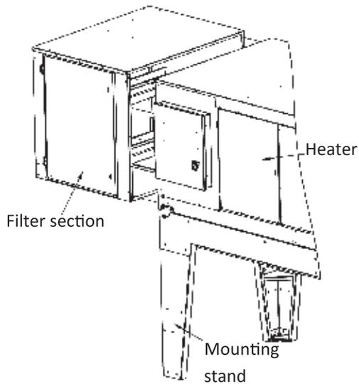
10. Using the 2 additional filter section support legs, brace, and provided fasteners to secure the filter section to the mounting stand legs at the inlet side.
