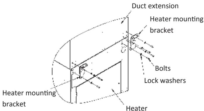
3. Continue attaching discharge accessories to the configuration as needed using the provided mounting brackets.
