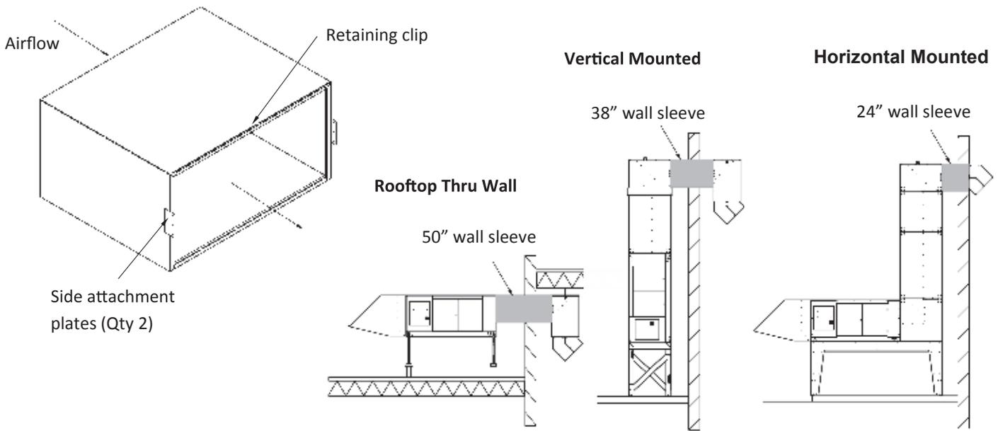
The S-Series wall sleeves (24", 38", and 50") are suitable for discharge duct work for either vertical or horizontal configurations. They are designed to be attached at its inlet side by a retaining clip and two side brackets. The discharge end is designed to hold either additional accessories by the same method (a retaining clip and two side brackets) or a set of directional elbows (page 50) and discharge collar. All wall sleeves are insulated to help mitigate noise and thermal losses.
