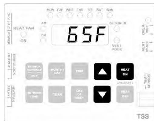
2. Press and hold the **HEAT OFF** button while pressing the **UP** or the **DOWN** button until the desired temperature for the heater to turn OFF is displayed.
