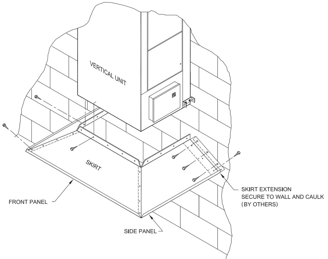
1. Attach the front panel of the inlet skirt to the unit top with the sheet metal screws provided.
