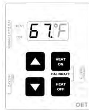
2. Pressing the **UP** or the **DOWN** button will display the current calibration difference above or below (-) the measured temperature.
