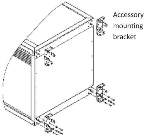
2. If heater is vertical downblast, remove the retaining clip and attach to the opposite flange. .
