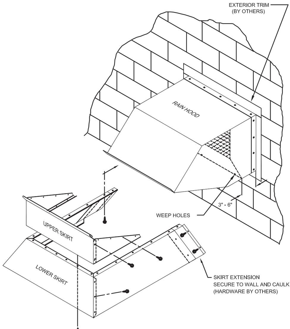
1. Assemble the upper skirt section with the sheet metal screws provided.
