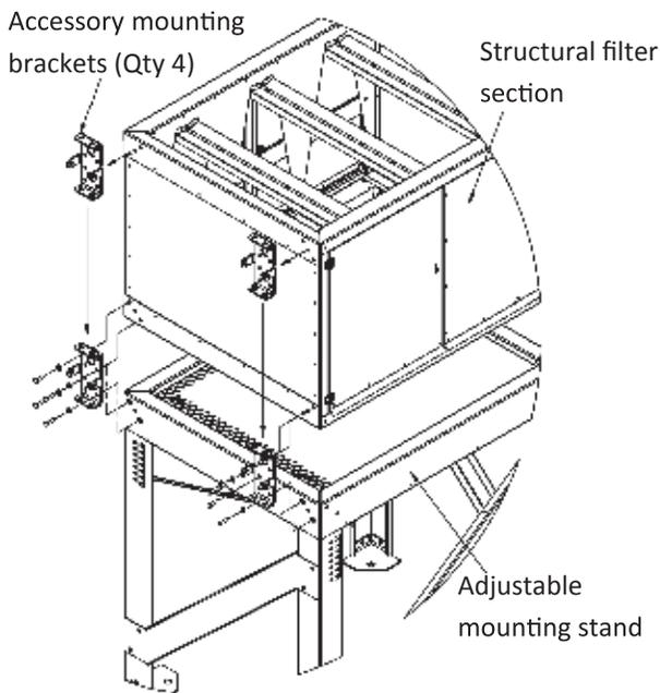
2. Lift the heater into place and secure by using 4 of the heater mounting brackets.
