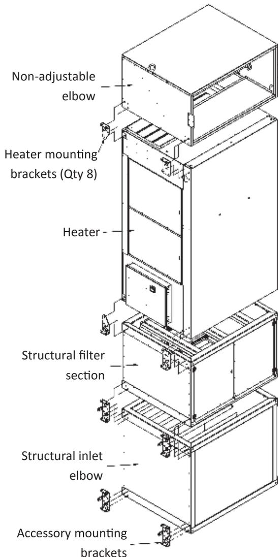
3. After having the configuration assembled, carefully lift entire assembled configuration into place and secure to the ceiling using threaded rod as directed by structural engineers.
