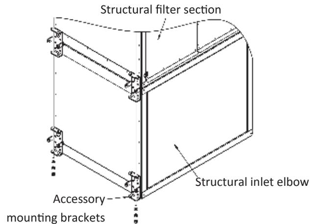
5. It is recommended to run support back to the wall to prevent swaying or tipping of heater and accessories.
