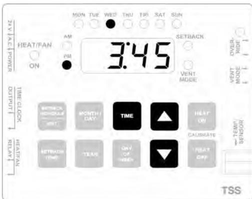
3. Press and hold the **MONTH/DAY** button while pressing the **UP** or the **DOWN** button until the current date is displayed.
