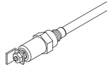
The flame rod senses the presence of flame and signals the flame safeguard relay. The presence of flame is detected by the flame rectification of the AC signal that is supplied to the flame rod thus creating the DC response. The resulting current flow produced can be measured with a DC microammeter. The reading should be steady and between 2.0 and 6.0 microamps ( $\mu\text{A}$ ).
