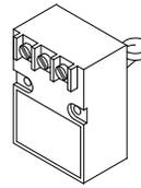
The DTS is mounted in the discharge of the heater. It senses the average discharge temperature and transmits a resistance signal back to the amplifier that corresponds to the discharge temperature.
