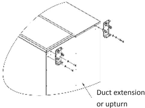
2. Place the duct extension on top of the existing installation and use the provided brackets to secure them together.
