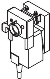
The damper motor operates on 24 Volts AC and switches power to the motor starter when the damper blades are fully open by the closure of the damper end switch. The damper end switch is an adjustable external auxiliary switch which has been factory set to operate when the damper is fully open. The damper motor will power closed when the heater cycles off. For detailed instructions refer to Damper Motor Replacement & Adjustment (page 89).
