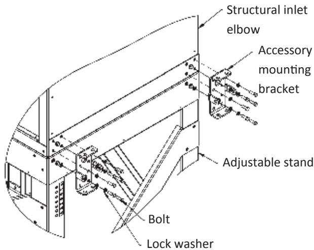
2. If filter section included, attach filter section to inlet elbow using the provided accessory mounting brackets. If filter section is not included, skip to step 3.
