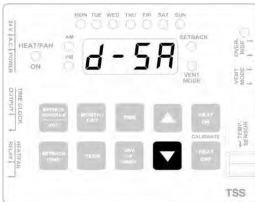
3. Press and hold the **YEAR** button while pressing the **UP** or the **DOWN** button to scroll to "YES" if daylight saving time should be recognized or "NO" if daylight saving time is not recognized.
