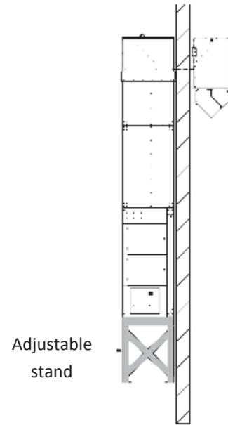
The Vertical S-Series Adjustable Stand is suitable for use in the up blast configuration in both indoor and outdoor locations. The 48" height is low enough so the control can may still be accessible without lifts or ladders, but high enough to avoid snow ingestion from the ground during winter months. The stand features 6" of adjustment (up to 54") and is suitable for applica-tions when you prefer the heater to be easily accessible for service, yet floor space or slab size may come at a premium.
