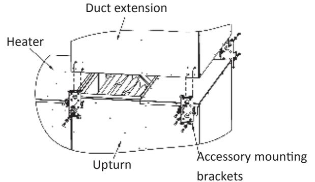
5. It is recommended to run support back to the wall to prevent swaying or tipping of heater and accessories. Use the provided mounting brackets to run threaded rod (by others) to support on walls (by others).
