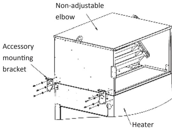
4. If not already done, remove the side attachment plates from the discharge end of the non-adjustable elbow. If attaching a discharge collar with directional elbows (page 50), also remove the retaining clip.
