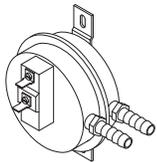
The airflow switch senses the pressure drop across the burner. It is factory set and not adjustable. It is designed to prevent burner operation if the airflow drops significantly below the minimum design airflow of the heater.
