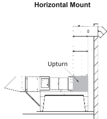
The S-Series upturn is suitable for supporting vertical discharge ductwork after turning airing 90° upward from a horizontal mounted unit. It is designed to be secured to the unit with the unit's retaining bracket and the upturn's threaded PEM studs. The vertical duct extensions are designed to be attached to the upturn with 4 accessory mounting brackets. Upturns are insulated to help mitigate noise and thermal losses.
