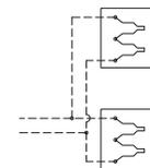
The TAS-2 option is used in conjunction with the RCS-S or TSS to average the space temperature between two distant points within a facility. It consists of four thermistors which are wired in
