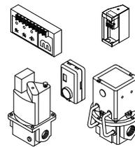
The EDSM temperature control system utilizes Maxitrol's Series 44 modulation controls. The Space Temperature Selector (STS) is set to the desired space temperature and it transmits a resistance output to the amplifier (AMP) to control the discharge temperature. The
