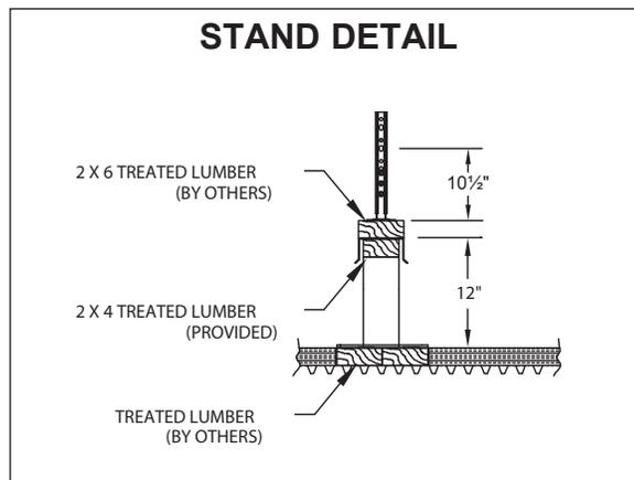
\* Dimensions allow for 1 1/2" clearance on each side
