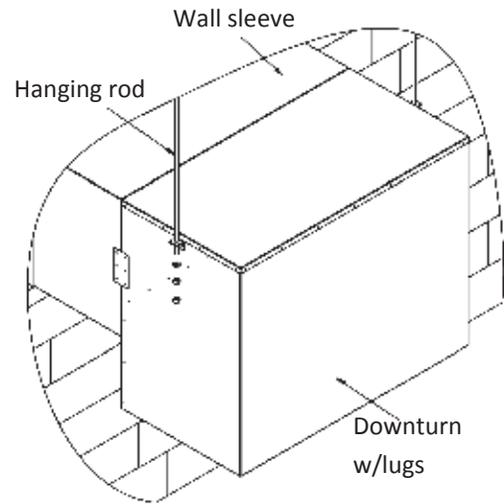
5. If attaching a discharge collar and directional elbows (page 50): Attach the discharge collar to the discharge face of the downturn with lugs and secure using self tapping screws. Arrange the directional elbows in the desired configuration before securing them to the discharge collar.
