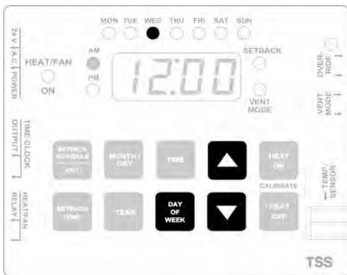
2. Press and hold the **TIME** button while pressing the **UP** or the **DOWN** button until the current time is displayed.
