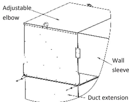
3. If not already done, remove the side attachment plates from the discharge end of the adjustable elbow. If attaching a discharge collar with directional elbows (page 50), also remove the retaining clip.
