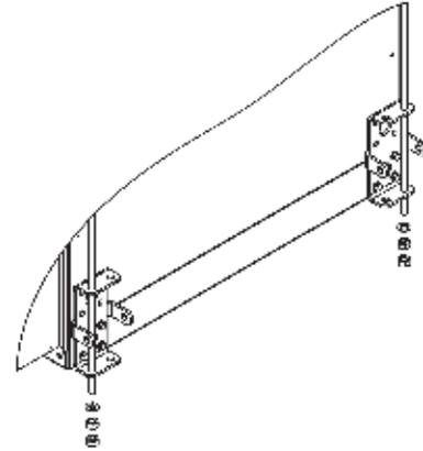
8. It is recommended to run support back to the wall to prevent swaying or tipping of heater and accessories.
