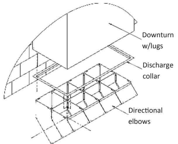
6. Seal all seams between accessories using appropriate contractor grade caulk to mitigate potential water ingestion and pressure loss.
