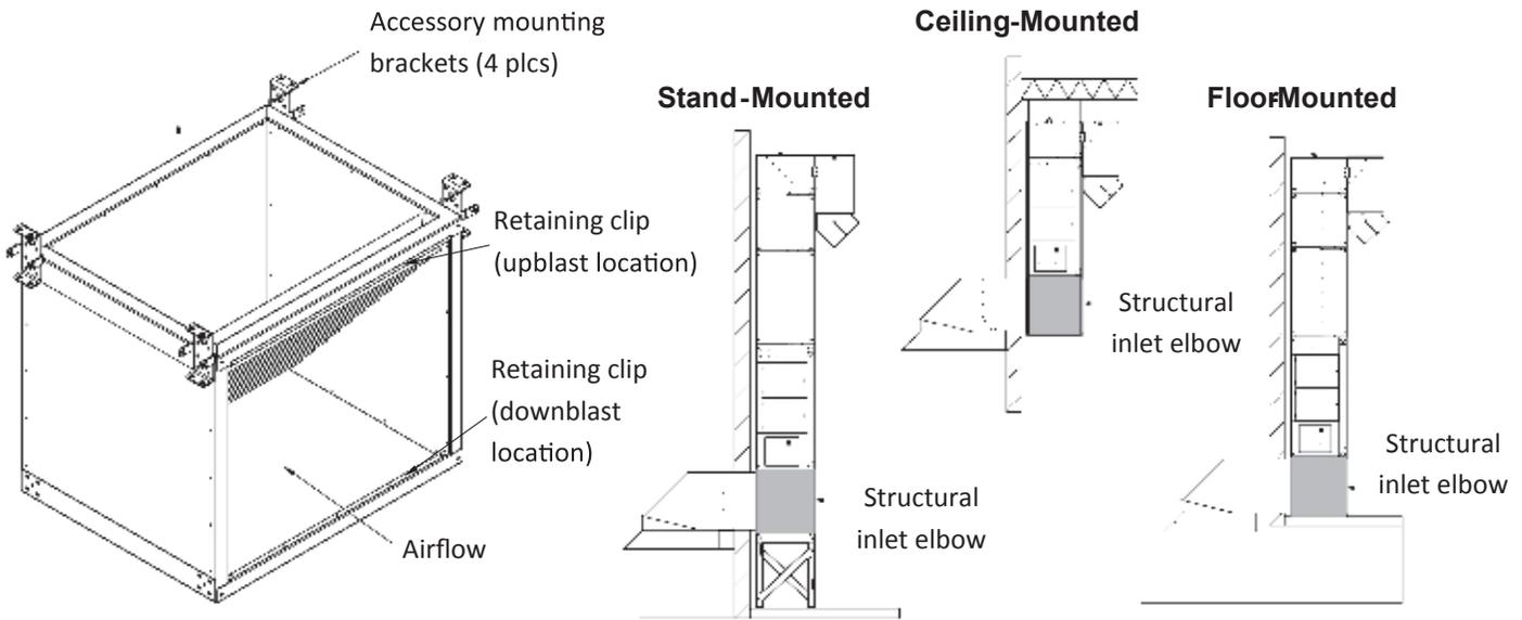
The vertical S-Series structural inlet elbow is suitable for indoor or outdoor use. The elbow has been structurally reinforced to support the weight of the unit and any additional accessories applicable to your installation. It can be used in floor-mounted applications, with or without a stand, as well as ceiling-mounted applications when hanging the unit with threaded rod. The elbow is insulated to prevent condensation and reduce noise levels.
