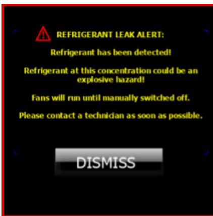
Figure. Alert will display on the HMI, warning the user of a detected leak.
