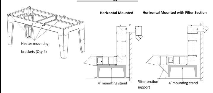
The horizontal S-Series mounting stand is suitable for outdoor pad mounted configurations. The 48" height is ideal for easy maintenance access while still remaining high enough to avoid potential snow ingestion from the ground during winter months. It is designed to be installed perpendicular to the building and includes room for both the unit and upturn to be situated on the frame. Additional support legs are provided if a filter section is ordered.
