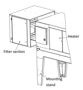
10. Using the 2 additional filter section support legs, brace, and provided fasteners to secure the filter section to the mounting stand legs at the inlet side.
