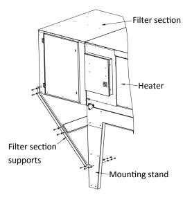
Seal all seams between accessories using appropriate contractor grade caulk to mitigate potential water ingestion and pressure loss.
