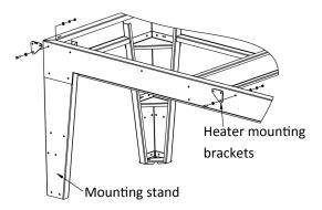
7. Set heater on stand and secure using the heater mounting brackets removed in the previous step.
