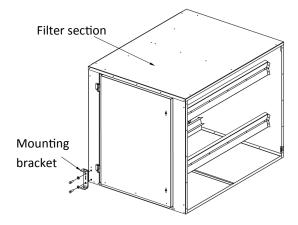
9. Lift the filter section into place at the inlet end of heater. Secure by resting filter section onto unit's retaining bracket while using self tapping screws to fasten the internal flange of the filter section the unit's front face.
