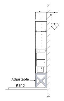
The Vertical S-Series Adjustable Stand is suitable for use in the up blast configuration in both indoor and outdoor locations. The 48" height is low enough so the control can may still be accessible without lifts or ladders, but high enough to avoid snow ingestion from the ground during winter months. The stand features 6" of adjustment (up to 54") and is suitable for applications when you prefer the heater to be easily accessible for service, yet floor space or slab size may come at a premium.
