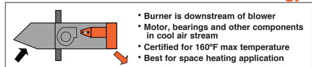
High temperature rise, Blow-Thru® Space Heaters are 40% to 70% more energy efficient than all other types of indirect and direct gas-fired systems used to heat/ventilate large commercial and industrial buildings. This has been documented by computer energy modeling and a growing list of over 300 on-site building studies.
